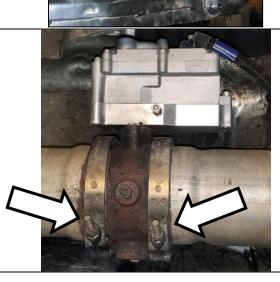
Weld the front adapter to the exhaust pipe. This weld must completely seal the exhaust system as it must retain pressure.
