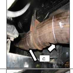
Cut out the marked pipe section using a reciprocating saw or cutting disk. Remove any burrs left on the edge of the pipe using a file or similar tool, then slide the pipe adapters onto the two cut ends of the pipe.
