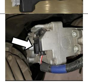
Lastly, route the harness with the black 4-pin connector down the firewall, along the frame rail to the exhaust brake actuator. Connect to the actuator and secure the harness along the frame.
