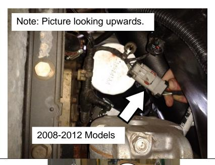
IMPORTANT Do not connect the harness to the EGR valve connector by mistake, it uses the same gray plug! Make sure the harness is connected to the VGT connector at the bottom of the motor.
